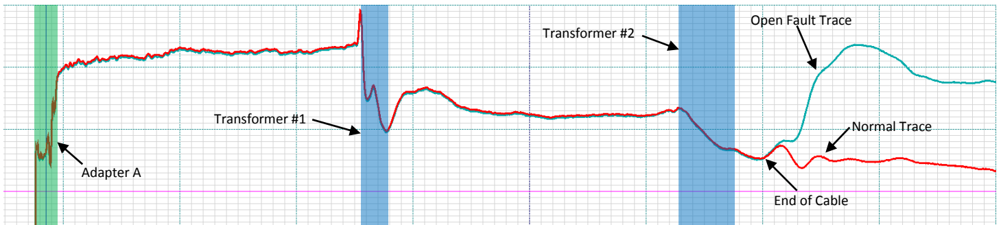
Figure 3 – Open conductor fault detection using Adapter A through two transformer couplings (transformers shown in shaded blue boxes)
