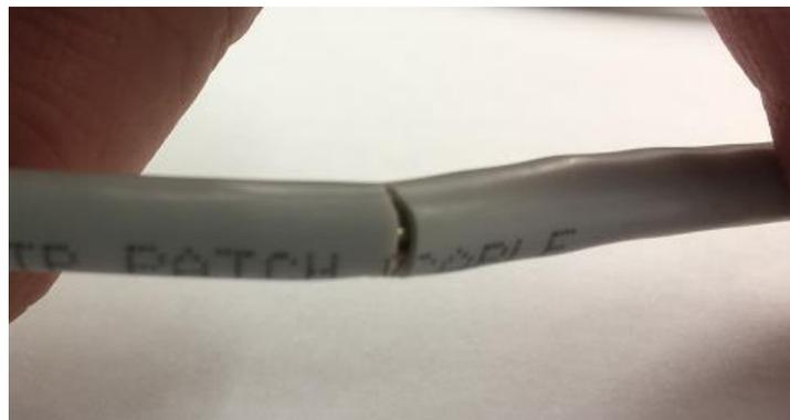
The cut in the cable sliced through two of the individual wires, affecting two of the wire pairs in the cable.
