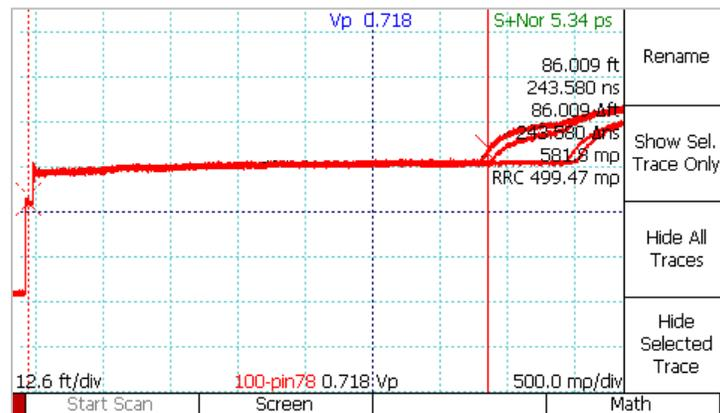
One wire in the 7-8 pin pair is also broken. Let's examine the cable at the 86 foot mark.
