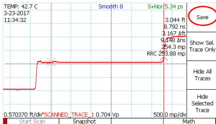
Enter a name for the saved scan. You use a USB keyboard or use the software keyboard that is built-in to the CT100B.
