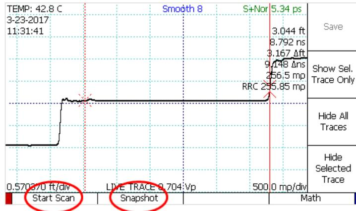
Once you have chosen a scan setting, press the Start Scan menu item to actually create your scan. This will create a red SCANNED TRACE superimposed on top of the live trace.
