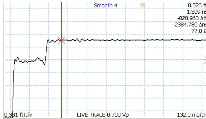
If we assume that the 77 ohms is a valid number, we should be able to go to end of the cable and define that as the correct value. The trace will then be redrawn using that assumption to mathematically adjust the readings as a function of the distance along the cable.
