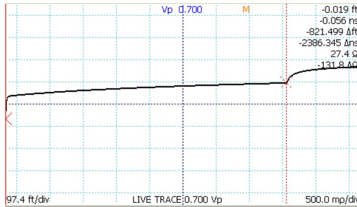
Note the continuous rise in the measured impedance. Yet, we know that there actually is no impedance change in the cable. The rise in the trace is an artifact of the measurement loss we see because of the difference between theory and practice.
