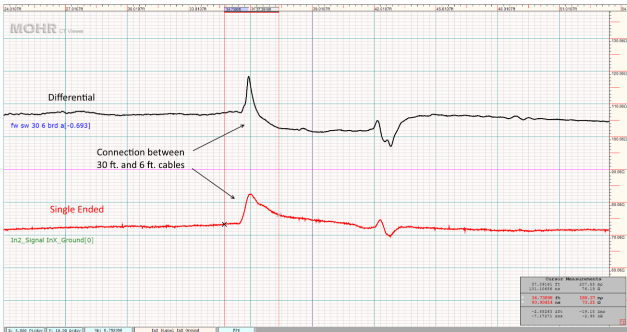
Figure 8 Comparison of a differential TDR trace to a single ended TDR trace using the setup of Firewire cables. On the single ended trace, note the elongated tail for the connection between the cables, the extra noise, and the grossly inaccurate impedance values
