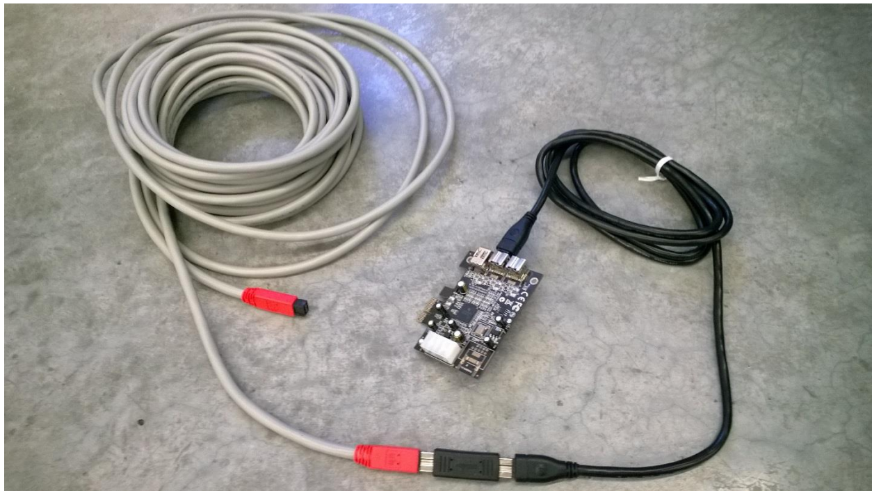
Figure 2 Test setup used for most of this document. A 30 foot cable is connected to a six foot cable, which terminates in a Firewire computer card. The test equipment, including the Mohr CT100B TDR and the Mohr TS-4 Adapter, are not shown.
