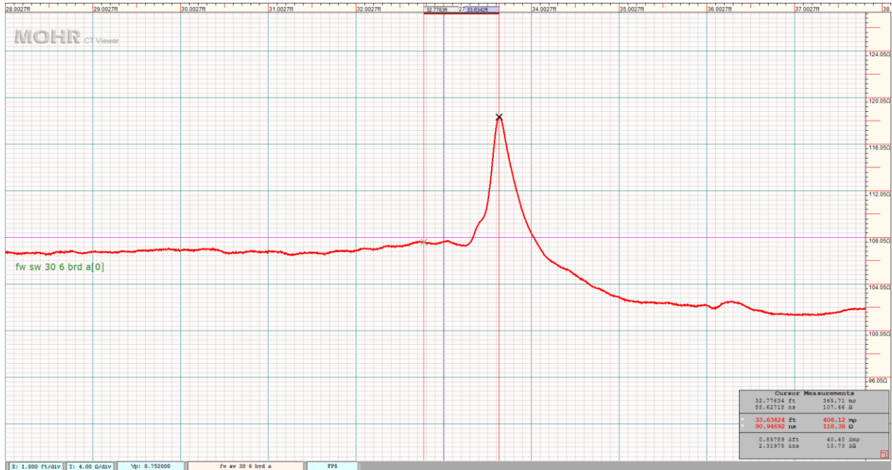
Figure 4 Reflection at connector between 30 ft and 6 ft cables. The height of the reflection is about 11 ohms above the baseline. A damaged or poor connector would have a bigger reflection.
