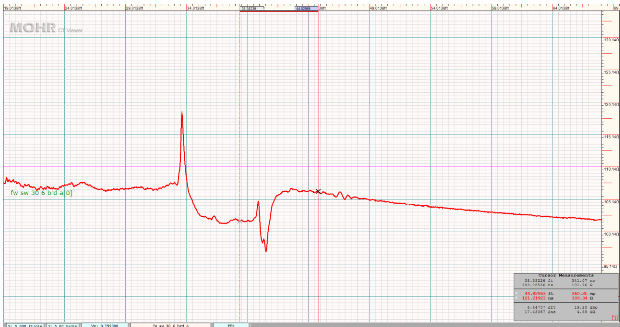
Figure 7 The region between the two cursors represents the end of the 6 ft. cable going through a connector into the termination in the computer card.
