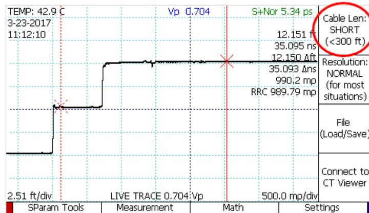
If you are not sure of the length, you can start with the short setting. Running Autofit (described below) will increase the length setting if necessary.
