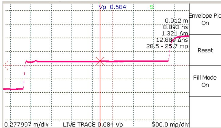
Now you can move or wiggle the cable to see if the connector is the cause of the intermittent fault. Sometimes this isn't possible, but you can just let the CT100B continue to record for long periods of time while waiting for the fault to occur.
