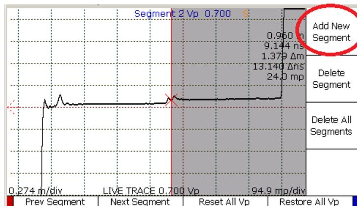
Now use the M-FUNCTION knob to set the Vp of the new segment. Note that as you turn the knob the trace is redrawn on the screen to reflect the new value. You can define additional segments as needed by positioning the cursor at the next joint and pressing Add New Segment again.
