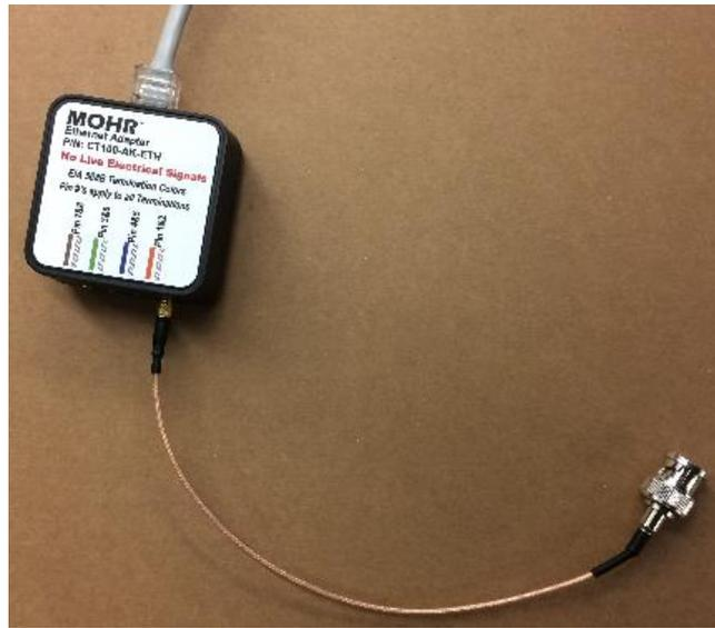
Our test cable is about 100 ft. long. After the cable has been connected to the CT100B, set the scanning resolution to *Normal* and the Cable Length to Short, and then use Autofit.<sup>1</sup> One of the cursors is now positioned approximately at the end of the cable.
