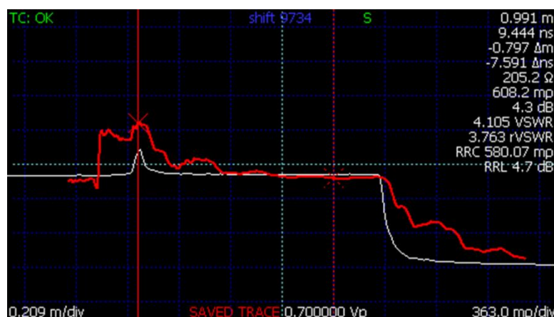
Figure 14: Clip lead adapter (red) and controlled-impedance adapter (white) testing of 3 ft. coaxial cable with short termination. Active cursor is at the test port. Clip lead adapters introduce severe TDR waveform distortion.
