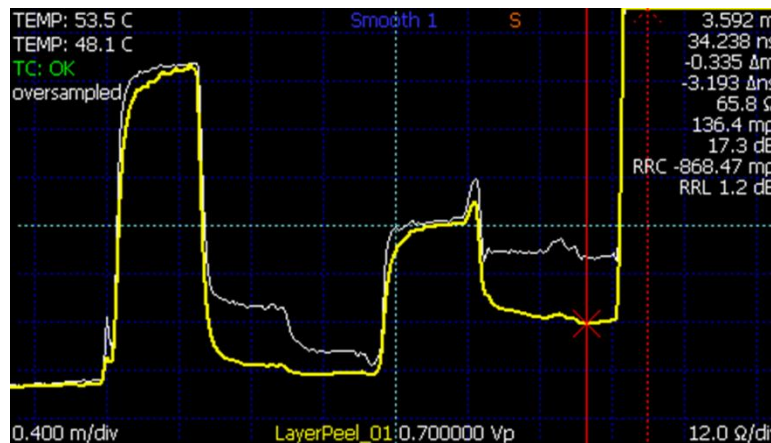
Figure 46: Example Layer Peeling trace (yellow) versus live TDR trace (white).
