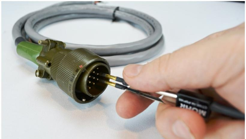
Figure 2: MOHR #16 Socket adapter testing a Mil-Spec Cable Assembly
