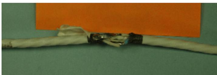
*Figure 4: Partial shield fault. The shield remained electrically contiguous with no significant DC resistance. The underlying twisted pair is undamaged.*
