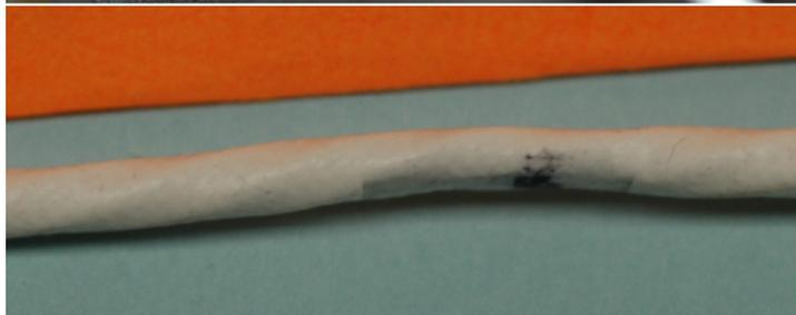
*Figure 3: Non-destructive clamp fault, causing deformation of the shield and underlying twisted-pair but no significant permanent damage following its removal. There would likely be no significant impairment of system performance.*
